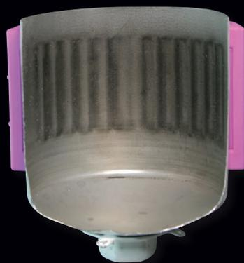
Photo of an actual cut-open filter, showing the debris trapped and held in the magnetic flux field of an AEROMAG, installed on a filter from a Lycoming IO540 for only 10 hours.
