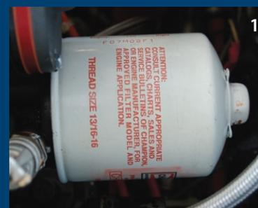
1 You don't have to wait until your next oil change to install AEROMAG™ because removal of the existing filter is not necessary. First, temporarily remove filter safety wire.
